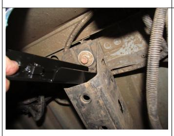
13. Place the double weld nut brackets into the rear of the chassis rails with the notch facing the outer rear corners of the vehicle.
