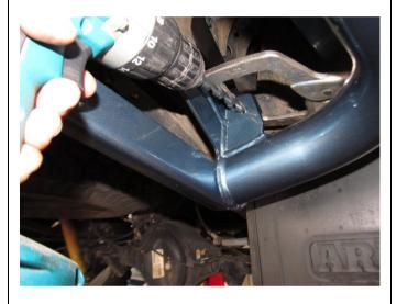
Using a drill with a Ø10mm drill bit, drill through the struts using the holes in the bar as quides.
