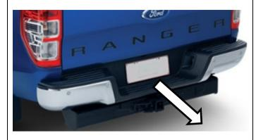
If either is fitted, remove the factory bumper bar and tow bar from the vehicle. If the vehicle has a tow wiring harness fitted, carefully place this to the side where it will not be damaged during fitment of the Rear Step Tow Bar (RSTB).
