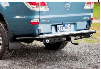
14. With the assistance of other people or a lifting device, lift the RSTB up on to the chassis rails aligning the holes in the bottom of the chassis with those in the verticle surfaces of the RSTB.
