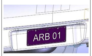
12. Fit the license plate to the license plate bracket using 2 M6 button head screws, 2 M6 washers and 2 M6 Flange nuts.
