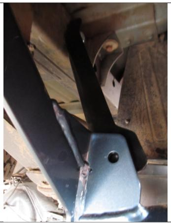
19. Attach the brace struts to the chassis using M12 x 1.75 (course pitch) bolts, M12 spring washers and M12 flat washers into the captive nuts directly in front of the spring hangers on each chassis rail.
