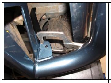
Use vise-grips, or a similar clamping device to hold the struts against the brackets on each side of the bar ensuring you have left access to the drill guide holes in the bar.
